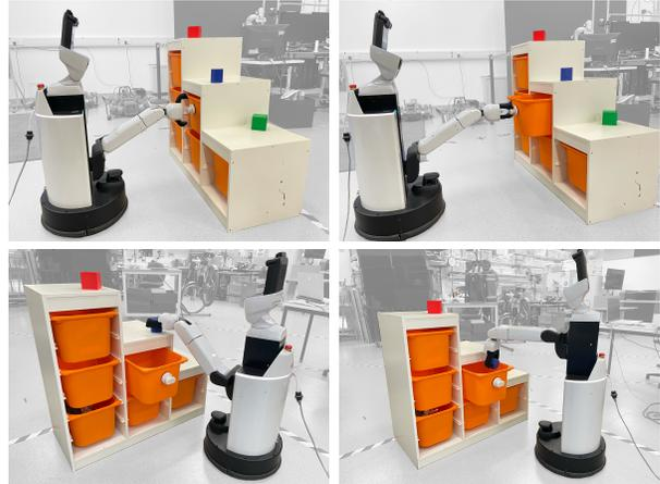
Fig. 1: Physical HSR performing R-LGP solution for table clearing task. The captured actions include grabbing knob, opening/closing drawer, picking object, dropping object.
